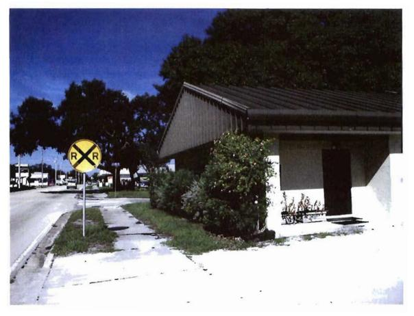
NORTH EAST SIDE OF BUILDING - WORK TO BE DONE: REPLACE PANELING, PAINT BUILDING, ADD ARCHITECTURAL ROOF AND ADD ASPHALT PAVING
